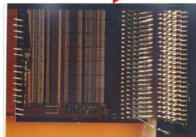
Microplex readout chip 128 channels, 47.5 \mu\text{m} pitch (Walker, Parker, Hyams)
