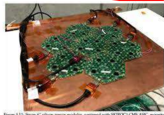
Figure 8.12: Seven 6" silicon sensor modules, equipped with SKIROC-CMS ASIC, mounted on a copper support (existing plane during the 2017 forward campaign).
